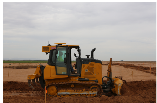
Figure 2 – Vector VR500 Smart Antenna installed on a bulldozer
