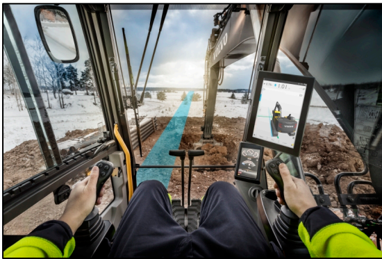
Figure 7 – Hemisphere GNSS-based technology is currently being used in Volvo CE's Dig-Assist solution
